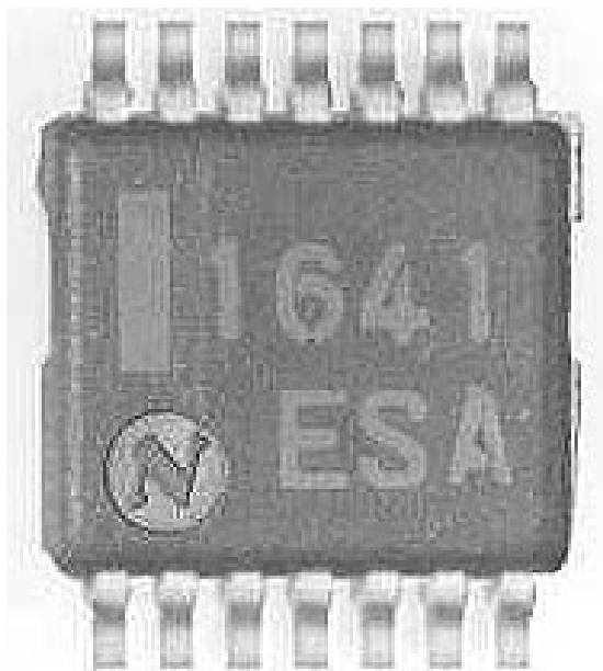
Fig. 4. Photograph of the mold package (package size: 6.2mm x 5.4mm).
